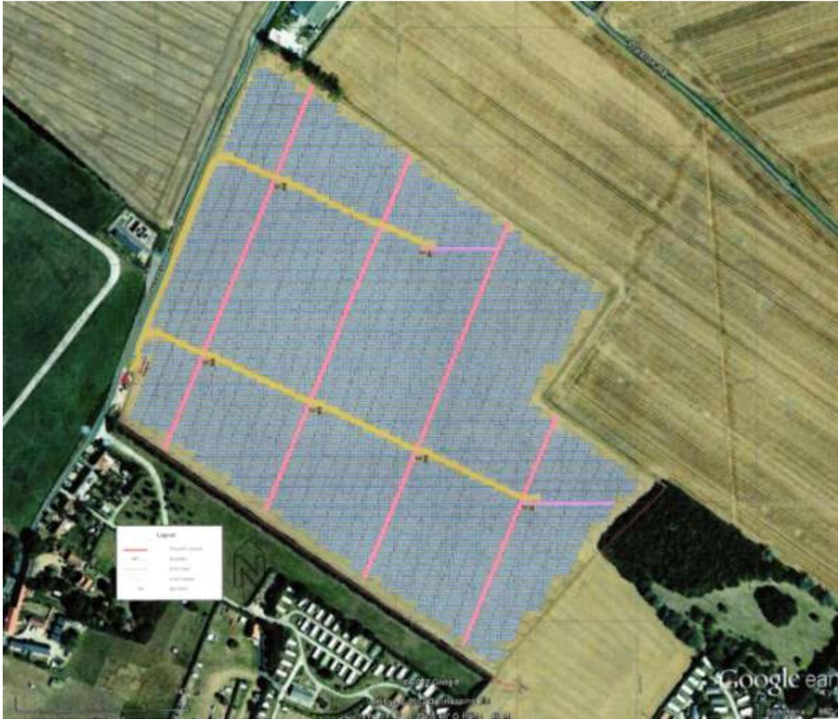
Fig. 2 Location of temporary access roads – in beige- and compound (south-west corner). Location of cable runs in pink.
